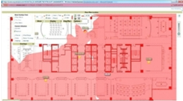
Figure 17: Channel Utilization in VisualRF (Interference)
